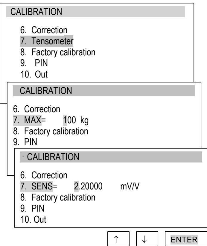
*Tensometer* option enables direct inscribing range (MAX) and sensitivity (SENS) of tensometric sensor by using navigation keys. Measurement range doesn't change.
