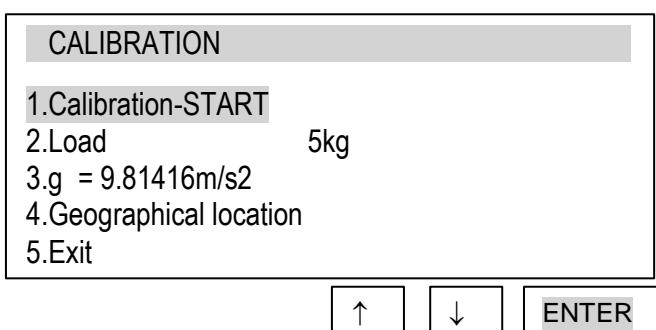
Use the navigation keys and *ENTER* to select *Calibration* and wait until the calibration process is completed.
