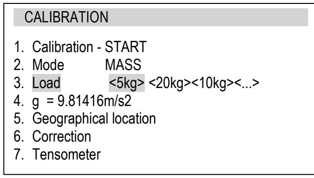
Use the navigation keys and *ENTER* to select *Calibration* and *Load*.
