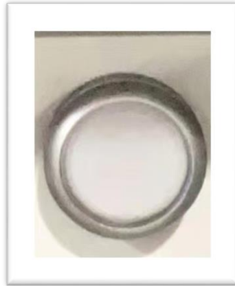
Logistics mode switch (pressed to open, not pressed to off)
