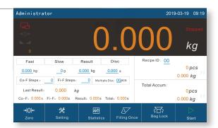
Calibration according to different materials with step hints to make the field calibration more convenient.
